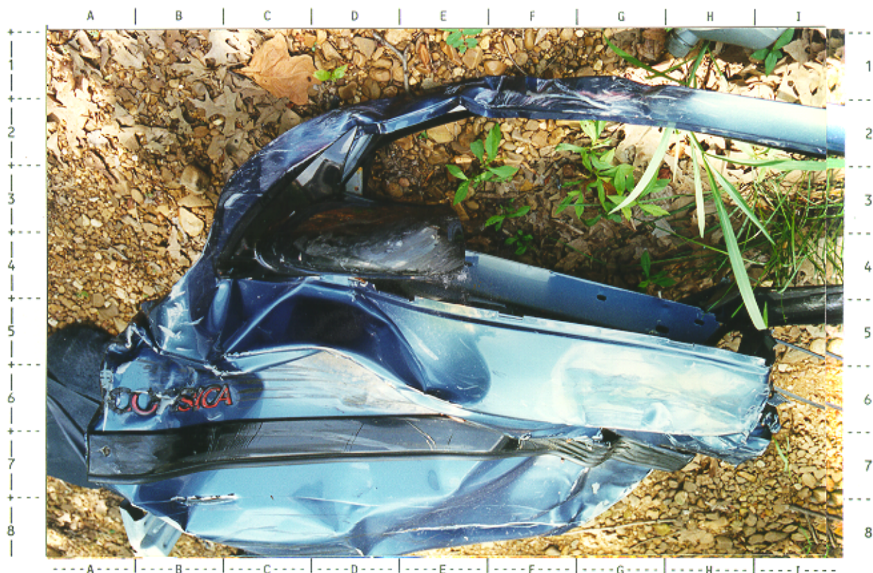
# 48 -- Damage to LF (driver's) door of 1991 Chevrolet; NOTE: red paint (1988 pickup's) transfer to top of window frame (cells G1--G2)
